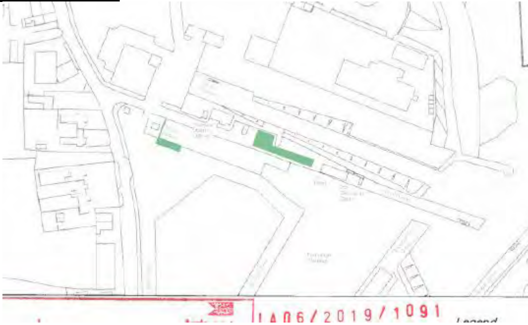
Drawing 02 showing the location of where the sound barriers will be positioned during dismantling works.
