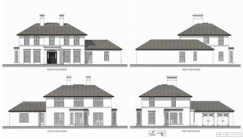
Figure 11: House A elevations
