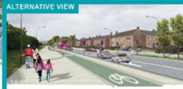
In areas where physical space is more limited, shared lanes may be required
