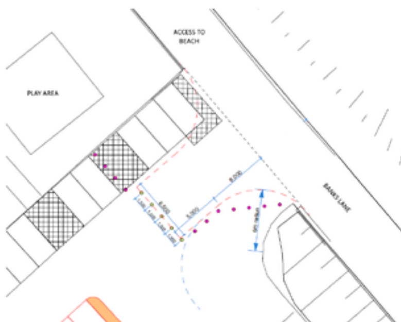
Image 2: Positioning of Bollards to create turning circle. Movable bollards shown in green, fixed bollards in purple.
