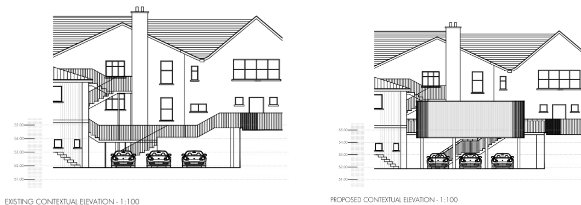
Figure 1: Existing and proposed elevations
