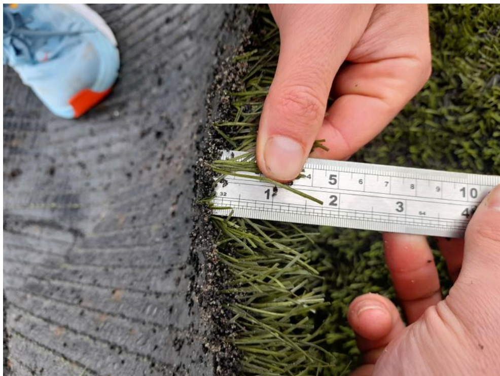
4 – Existing 3G Synthetic Turf (50mm)
