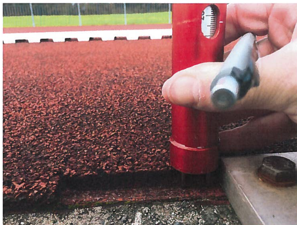
Thickness of track in exposed area. Note the track is cut and is thicker than reading of probe
