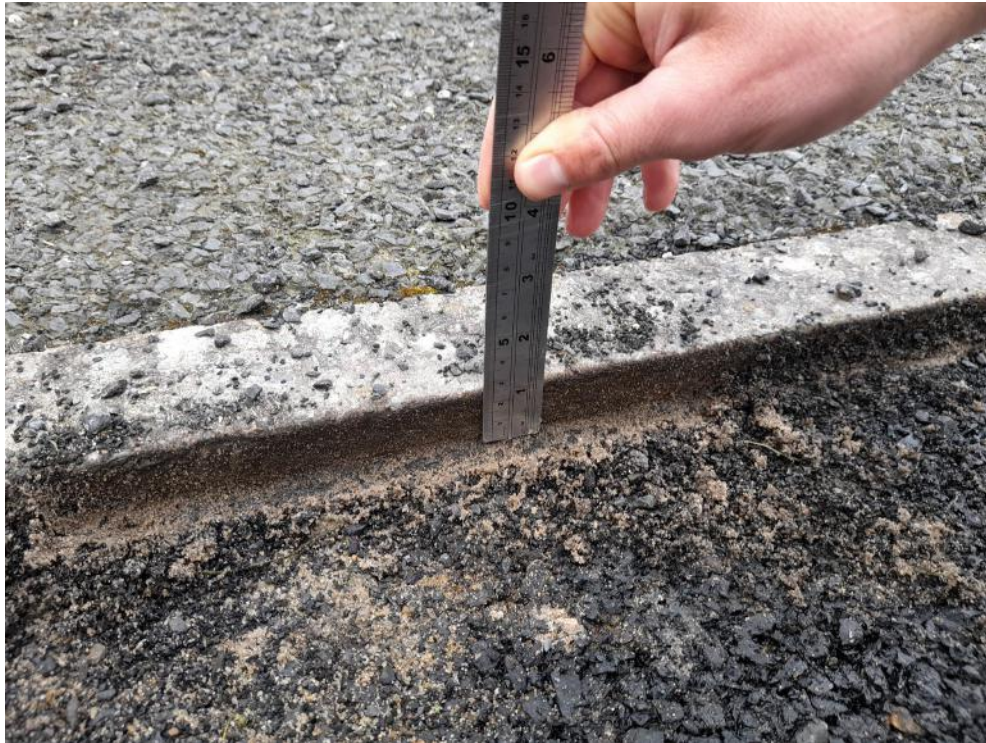
3 – Depth to Engineered Base Layer
