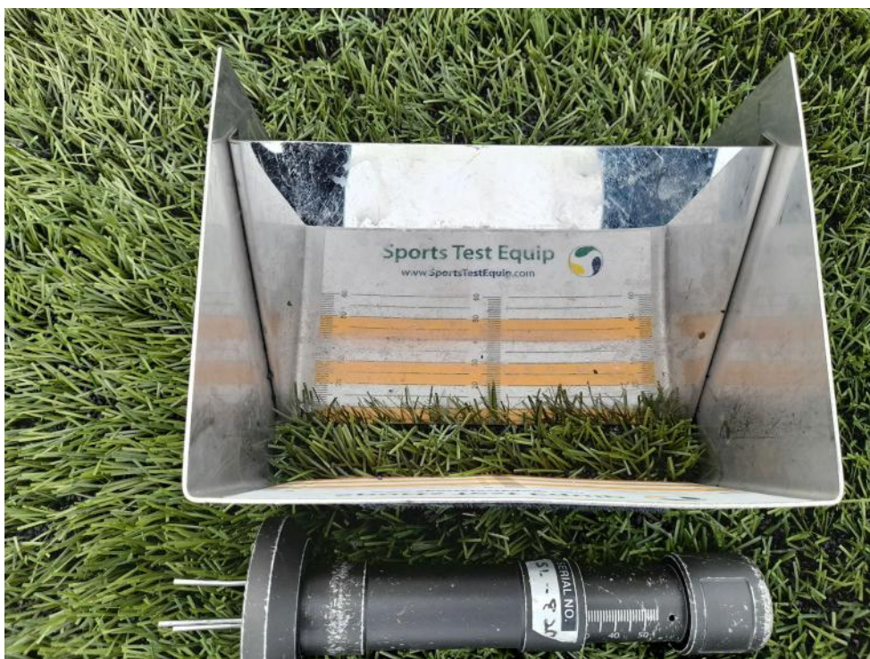
10 – Pitch Free Pile Height and Infill Depth
